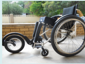
The free wheel is used to accommodate the tough and sandy terrain in Botswana.
